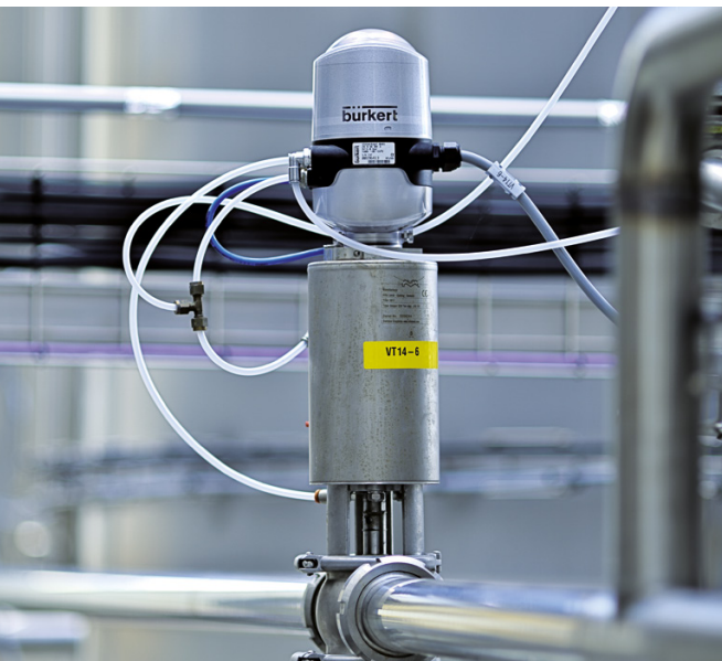
Flow management is ensured by agrifoodstuff valves, controlled by fieldbus
