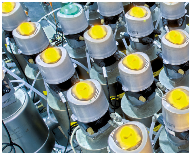
The series 8681 control head can be used on every type of valve from different suppliers.
